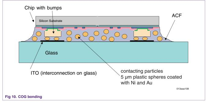
The following parameters apply to all COG bonding (Au bumps) processes:
