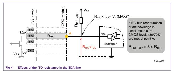
For this reason the SDA signal in LCD driver ICs is sometimes split into SDAIN and SDAOUT. A number of possibilities for connecting LCD to the host micro exist, three examples are given.
